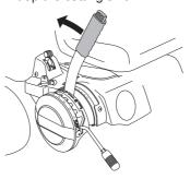
7 Push the unit in so that the interior plugs touch the bottom of the equipment frame's grooves.
